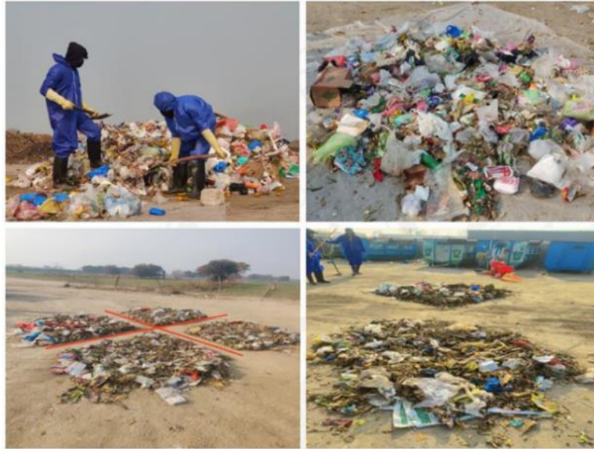
Figure 3: Coning and Quartering of the Municipal Solid Waste
